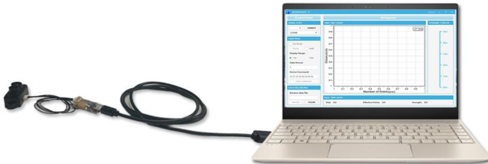
Figure 4 Schematic Diagram of Correct Connection
